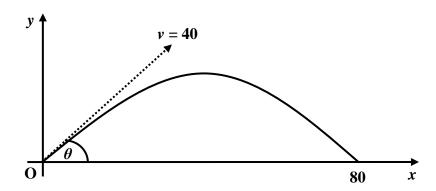
An arrow fired from ground level at a velocity of 40 m/s, is to strike the ground 80 metres away as shown in the diagram above.
