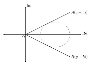
Consider a cubic polynomial y = P(x) with real coefficients and roots 0,  $q \pm hi$  where q and h are real and h > 0. In the diagram above, the roots form the vertices of an isosceles triangle OAB in the complex plane. The roots of P'(x) = 0 are the foci of the sketched ellipse which touches the triangle at q + 0i. We have sketched the case q > 0 and with major axis lying on the real axis. The centre of the ellipse is NOT the origin.
