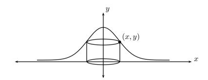
The volume of the cylindrical shell  $dV = 2\pi xydx$ . Total volume is
