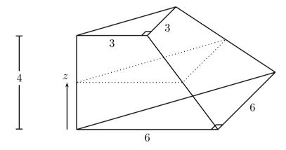
The base and top of the solid depicted are right angled isosceles triangles. A pupil is required to determine the volume by slicing parallel to the base. A typical slice parallel to the base at height z from the base is marked.
